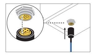
The other end of the cable has two connectors, one male and one female.
